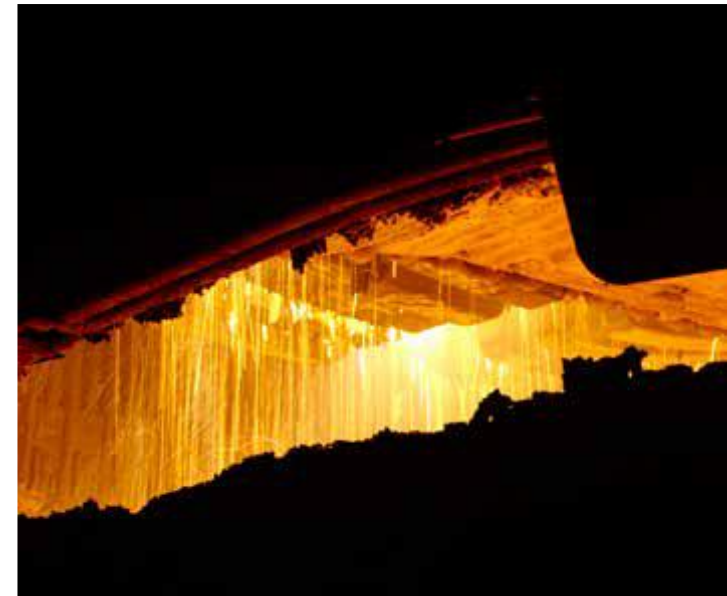
Preheated steel on the finger system
